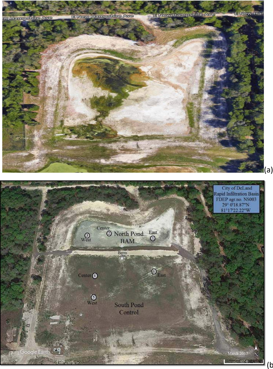
Figure 4 Aerial Photographs of (a) North (pre-study) RIB without separation berm and (b) BAM RIB (North) and Control RIB (South) with Lysimeter Locations Source: Google Maps (reference time is May 2016 and March 2017)
