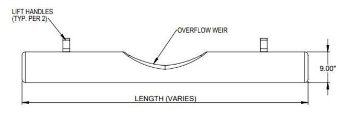
NOTE: PERIODIC MAINTENANCE SHALL INCLUDE CLEANING GUTTER EEL SURFACE WITH HIGH PRESSURE WASH OR BRUSHING SURFACE WITH BROOM.
