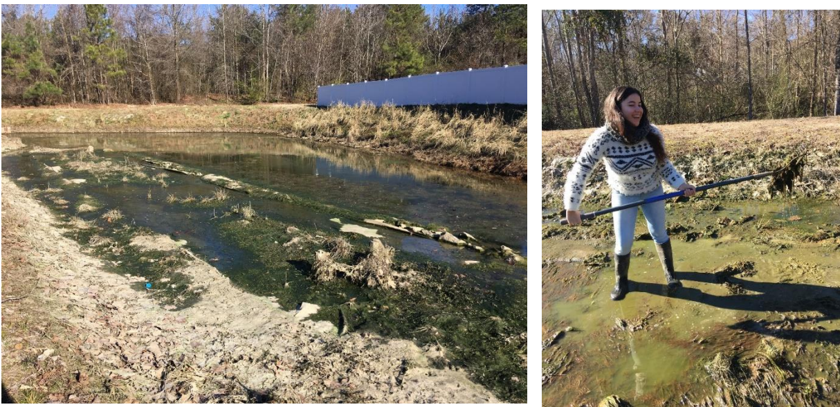
Figure 17. Clogging of the Bridgewood filter with biological material (left) and restoring infiltration by removing and raking the filter (right).
