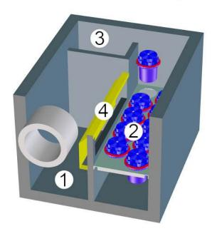
Chamber 1: Pretreatment Chamber – Untreated water enters the StormSafe here
