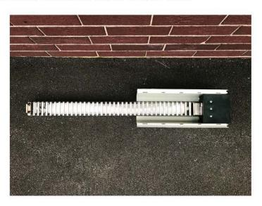
Fabco's Trench Drain Filters are comprised of one or more perforated metal square tubes called debris shields and a bypass hood assembly. The 4' long debris shield is comprised of a perforated stainless steel screen which keeps coarse material out of the filter, and a replaceable filter media product for treating the water. The system can accept one of two treatment media types: Oil/Grease and Phosphates/Nutrients.
