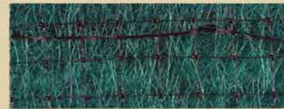
Western Excelsior's permanent turf reinforcement mats are composed of 100% synthetic components. A matrix of green or tan polypropylene fibers is mechanically bound (stitched) between two UV stabilized heavy-duty synthetic nets. Each is a permanent rolled erosion control product that provides short-term erosion protection and long-term turf reinforcement for greater than 36 months.
