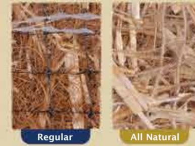
Excel CS-3 is an Extended-Term ECB comprised of a blended matrix of 70% certified weed free agricultural straw and 30% clean coconut. The blended matrix is mechanically (stitch) bound on two inch centers to Regular or All Natural netting. Excel CS-3 offers extended longevity, compared to straw matrix ECBs, thus providing a longer lasting alternative for moderate gradient slopes and channels.
