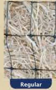
All of Western Excelsior's Long-Term products are manufactured in a double net configuration and consist of an organic matrix intended to degrade over time. Coconut or Excelsior fibers are utilized as matrix materials, providing erosion protection and mulching for a period greater than 24 and up to 36 months. Heavy duty, UV stabilized netting is exclusively utilized for regular, long-term products. Coconut blankets are also available with All Natural netting.
