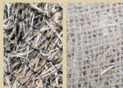
Aspen Excelsior Logs consist of a machine-produced high-altitude Rocky Mountain aspen excelsior matrix confined by a synthetic, tubular net to form a log of specific length, mass and diameter. Excel Aspen Excelsior Logs are designed to reduce hydraulic energy and filter sediment-laden flow in channels and on slopes. The logs are flexible, to conform to soil surfaces, and are secured by staking to create a temporary water-permeable structure.
