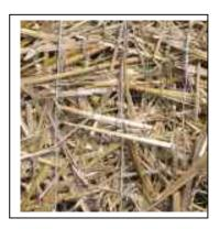
**WinterStraw™** Single Net Products are short term, single top net erosion control blankets that are machine-assembled using 100% agricultural straw fibers. The straw fibers are evenly distributed throughout the entire area of the blanket to a rough thickness of 3/8″ and stitched to your choice of netting using high strength degradable thread. Biodegradable thread is used on our Bio (Jute) products.
