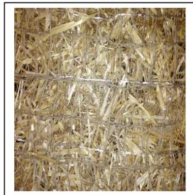
**WintersChoice™** Products are extended-term, double net erosion control blankets that are machine-assembled using a blend of 70% agricultural straw and 30% coconut fibers. These fibers are evenly distributed throughout the entire area of the blanket to a rough thickness of 1/2" and stitched between biodegradable jute netting using biodegradable cotton thread. Biodegradable thread is used on all of our Bio (Jute) products.
