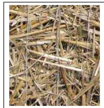
**WinterStraw™ HV** (High Velocity) Double Net Products are short term, single top & single bottom net erosion control blankets that are machine-assembled using 100% agricultural straw fibers. The straw fibers are evenly distributed across the entire area of the blanket to a rough thickness of 3/8" and stitched between your choice of netting using high strength degradable thread. Biodegradable thread is used on our Bio (Jute) Products
