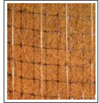
**WintersCoir™** Products are long term, double net erosion control blankets that are machine-assembled using 100% coconut fibers. These fibers are evenly distributed throughout the entire area of the blanket to a rough thickness of 3/8" and stitched to your choice of netting using high strength degradable thread. Biodegradable thread is used on our Bio (Jute) products.
