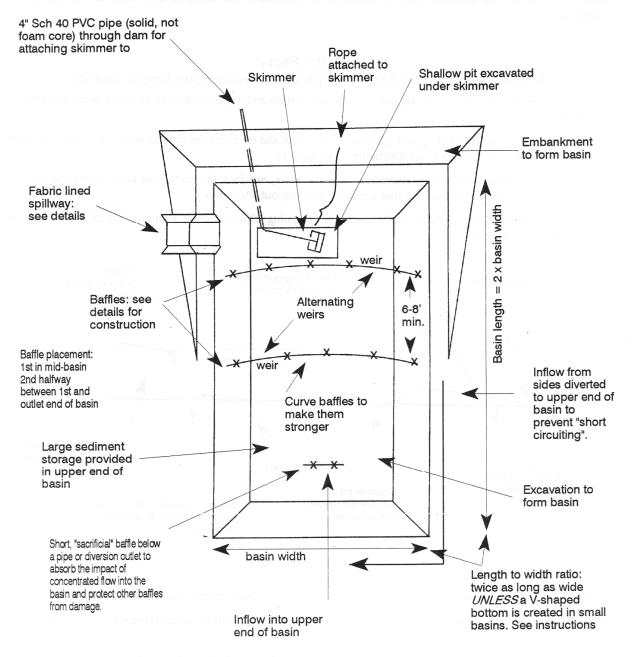
NOTE ON SPILLWAY PLACEMENT: Whenever possible place the spillway around one end of the dam instead of in the fill for the dam to minimize the chance of failure. Care must be taken when the spillway is in fill to follow the installation instructions and keep outflow on the fabric lining and off the erodible fill.
