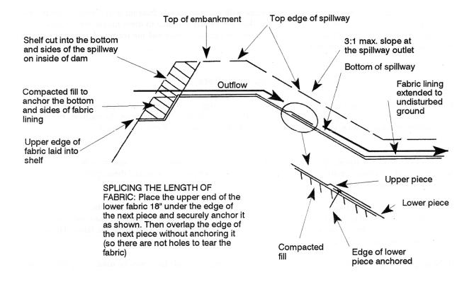
This type of spillway can only be used where there is an appropriate location. Topography, property lines, and other factors may require the use of a riser and barrel even in basins with small catchments.
