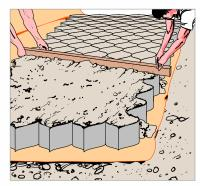
Install GEOWEB® layers as specified. Assure minimum 2 inch (50 mm) set back.
