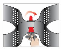
5 Cut GEOWEB® front fascia panels with utility knife to insert ATRA® keys.
