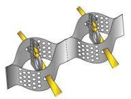
Figure 9 ATRA® Tendon Clips with Tendons through the Geoweb Cell Wall.
