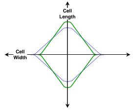
Figure 1 Variable Expansion of the Geoweb Cell
