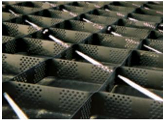
The GEOWEB® system may be designed as a protective cover over impervious geomembranes to prevent damage and degradation. GEOWEB® liner protection is a 'complete solution' including integral tendons and ATRA® tendon load transfer clips to create a suspended support system with selected infill. By confining infill in the GEOWEB® system, slopes can be designed steeper while still maintaining strength and integrity of the liner.
