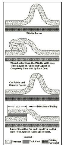
and maneuvering of equipment on the paving fabric. Wrinkles that result in three layers of fabric should be repaired. Generally, these wrinkles will be more than 1" high. They should be slit and laid flat in the direction of paving.. Wrinkles less than 1" high are usually not a problem and can be left in place.
