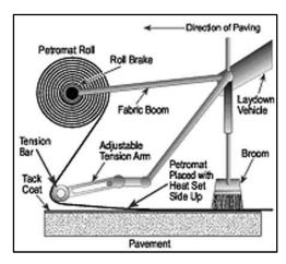
laydown equipment may also have a tension bar to apply the paving fabric smoothly and keep wind from rolling up the edges of the fabric as it is laid. The tension bar can often be adjusted as needed to smooth out the paving fabric. Best results may be obtained if this bar is bowed out.
