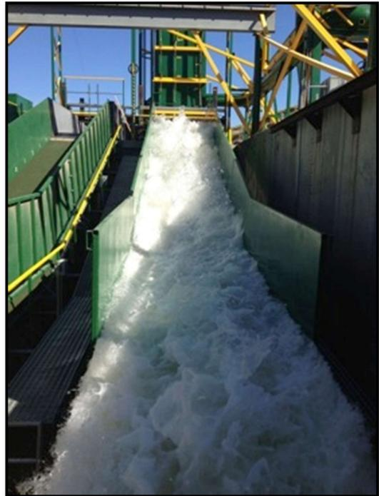
**Figure 7. HydroTurf® Wave Overtopping Testing at CSU**
