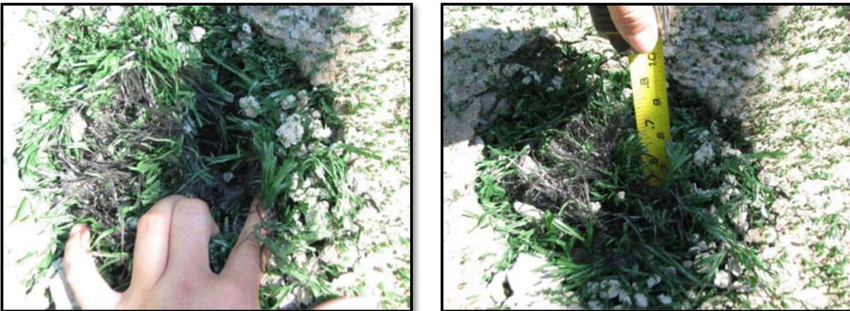
**Figure 6. Intentional Damage Simulating a Large Hole through HydroTurf®**
