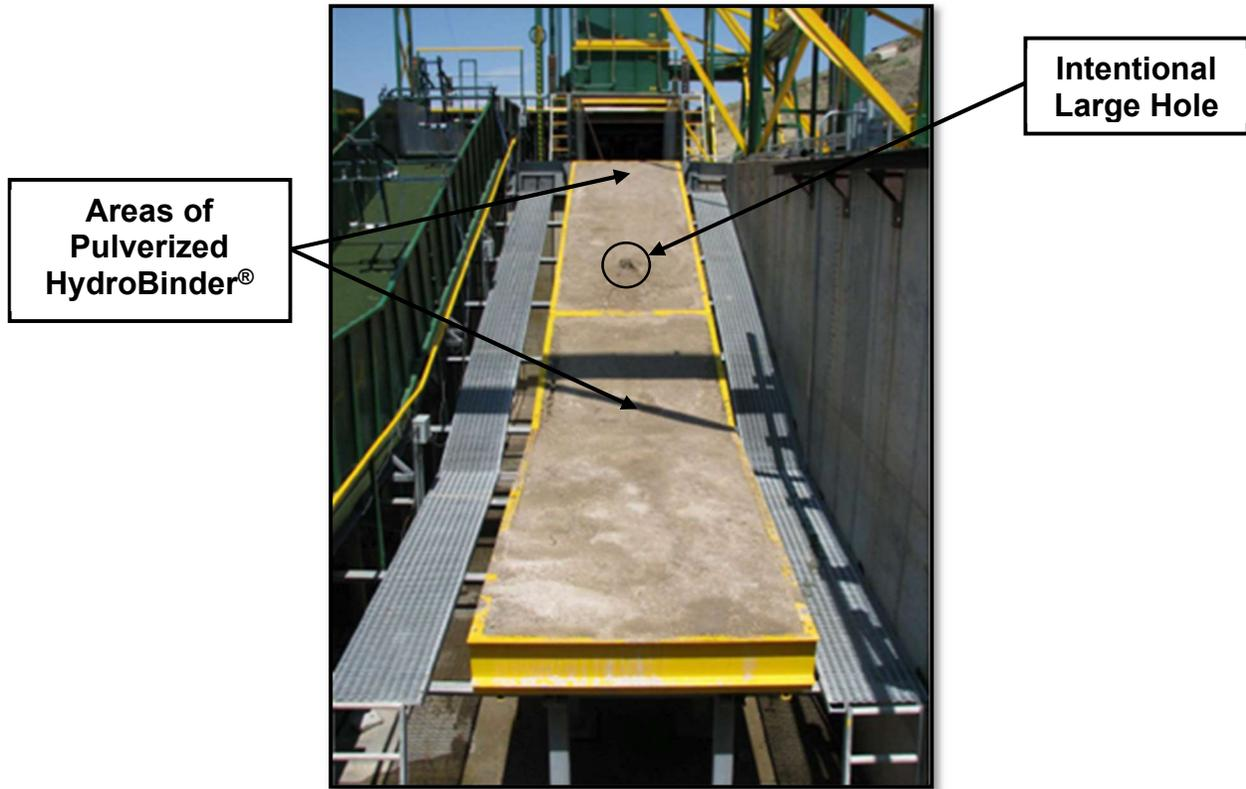
**Figure 9. Highly Erodible Silty Sand Subgrade upon Completion of Wave Overtopping Testing**
