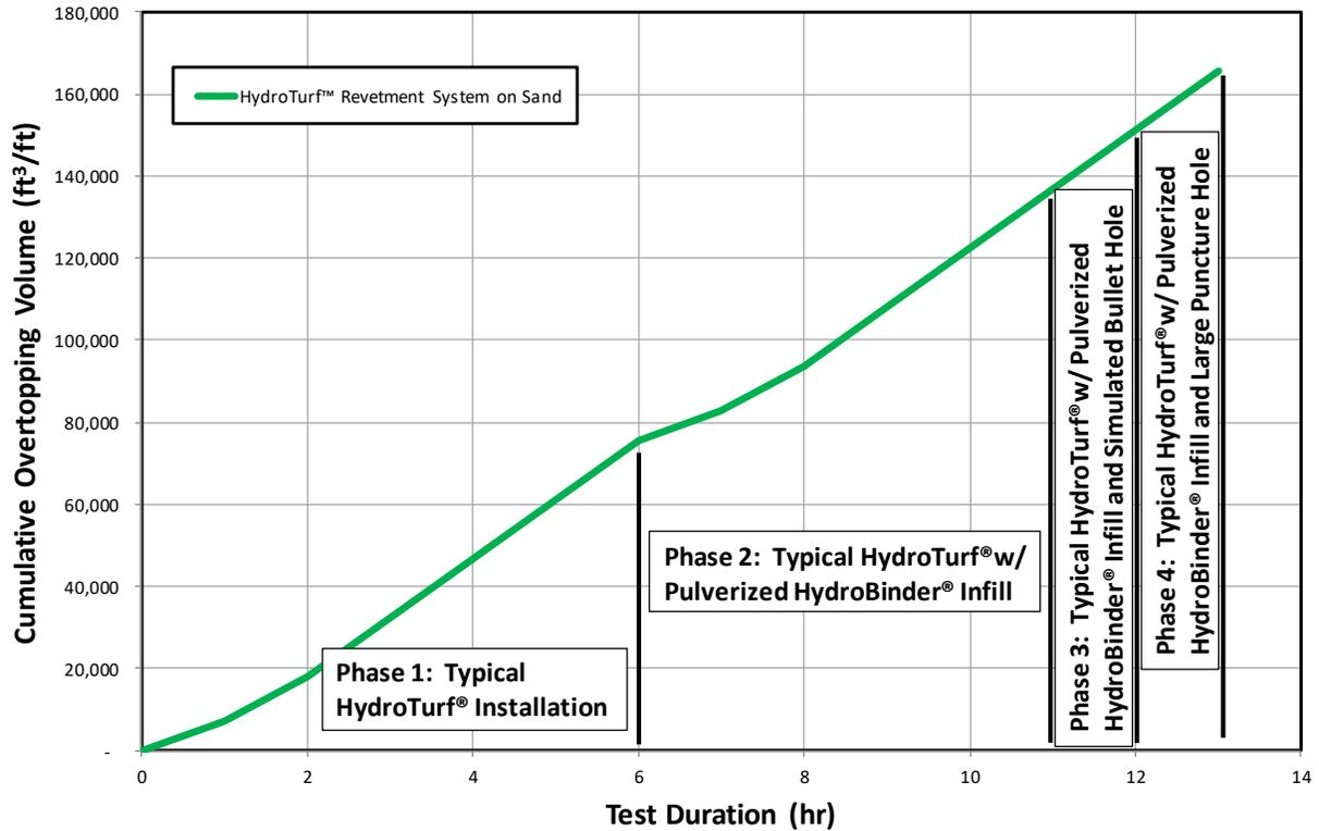
**Figure 10. HydroTurf® Cumulative Wave Overtopping Volume Progression**
