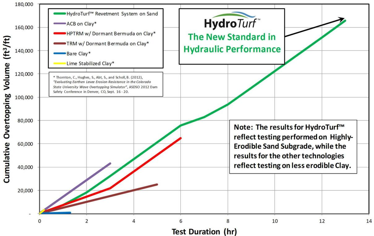
**Figure 11. Armoring Performance for Levee Landward-Side Protection from Wave Overtopping**
