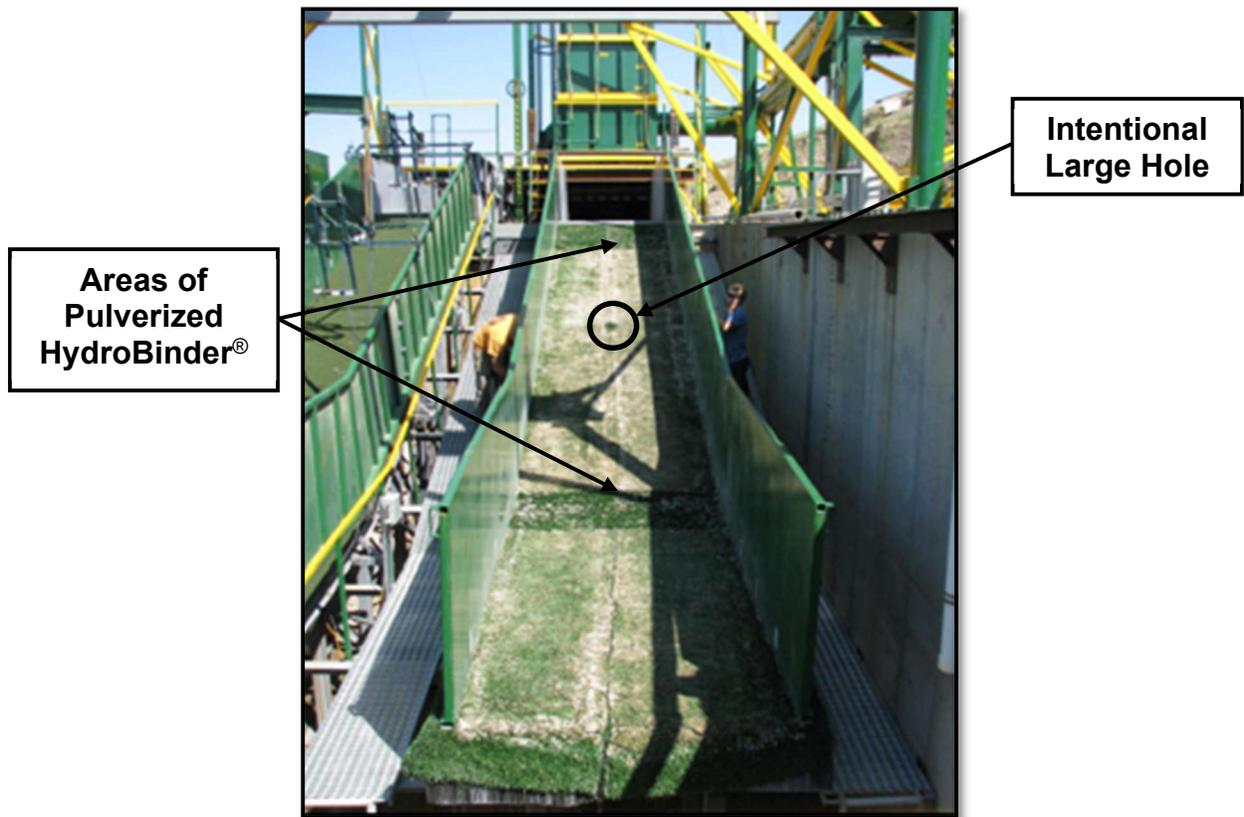
Figure 8. HydroTurf<sup>®</sup> System upon Completion of Wave Overtopping Testing
