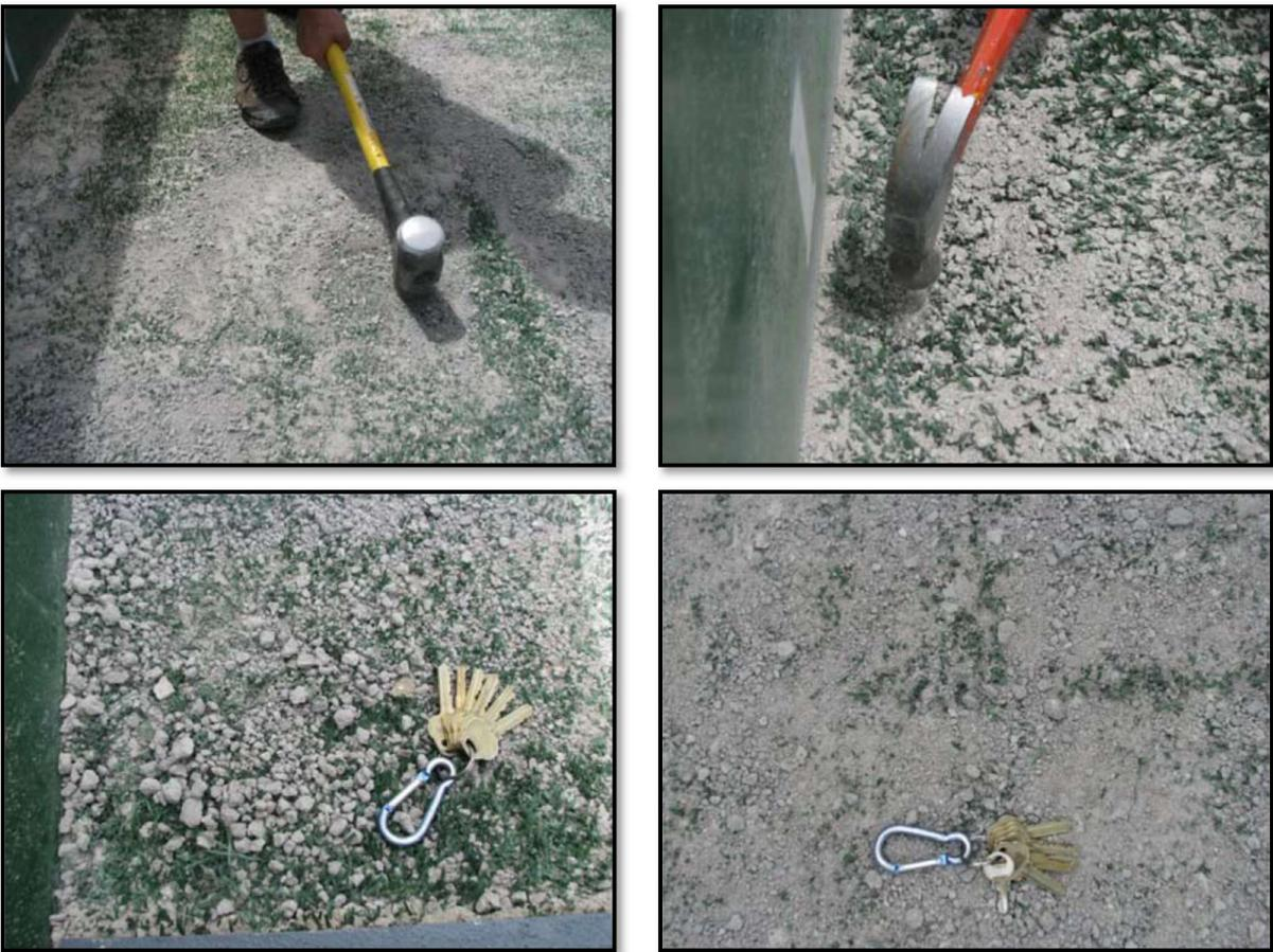
**Figure 4. Intentional Damage by Pulverization of HydroBinder® Infill**
