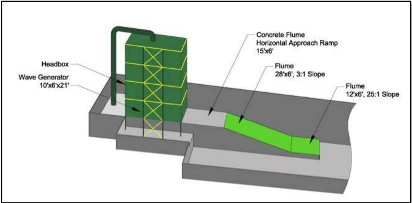
**Figure 1. CSU Wave Overtopping Test Facility Diagram**
