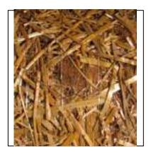
WintersChoice<sup>™</sup> Products are extended-term, double net erosion control blankets that are machine-assembled using a blend of 70% agricultural straw and 30% coconut fibers. These fibers are evenly distributed throughout the entire area of the blanket to a rough thickness of 3/8″ and stitched to your choice of netting using high strength degradable thread. Biodegradable thread is used on our Bio (Jute) products.
