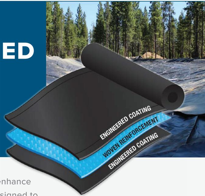
A heavyweight fabric incorporating a special weave pattern to enhance puncture, flatness, and tear properties. The coating recipe is designed to improve toughness and abrasion resistance. This product is intended for exposed applications up to 10 years.
