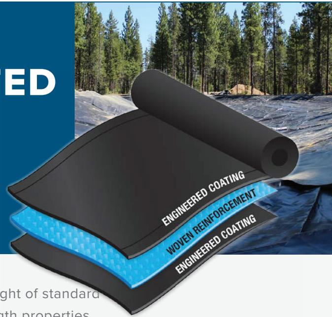
A heavyweight, reinforced polyethylene material with ½ the weight of standard 40 mil non-reinforced HDPE, but with double the physical strength properties. The coating recipe is designed to improve toughness and abrasion resistance. This product is intended for exposed applications up to 15 years.
