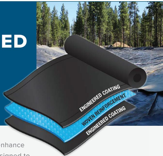
A heavyweight fabric incorporating a special weave pattern to enhance puncture, flatness, and tear properties. The coating recipe is designed to improve toughness and abrasion resistance. This product is intended for exposed applications up to 5 years.
